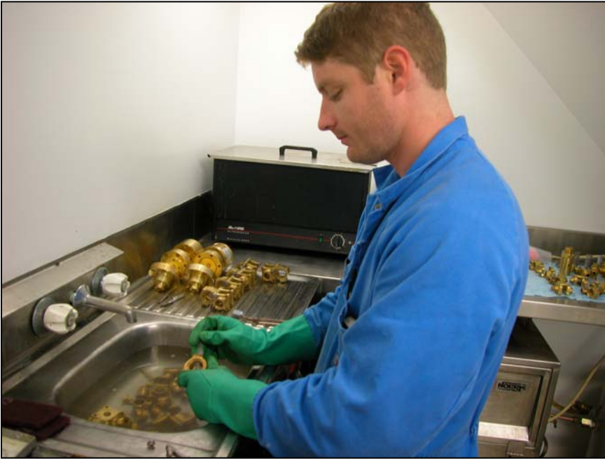
Pre-cleaning oxygen handling components
