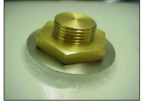
SPARE PENETRATORS (with brass "O" ring blanking bolt)
