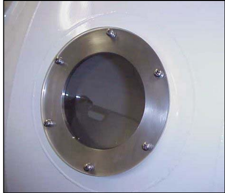
MANWAY & VIEWPORT FORGINGS (designed with lips to ensure 100% x-ray of welds)
