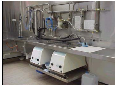
CLEANING (all gas carrying components are cleaned to US Mil Standard 1330D)
