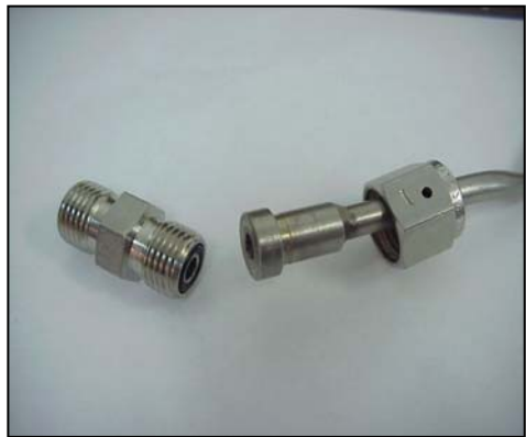
PIPEWORK (stainless steel tubes welded with VCO "O" ring seal Cajon fittings)
